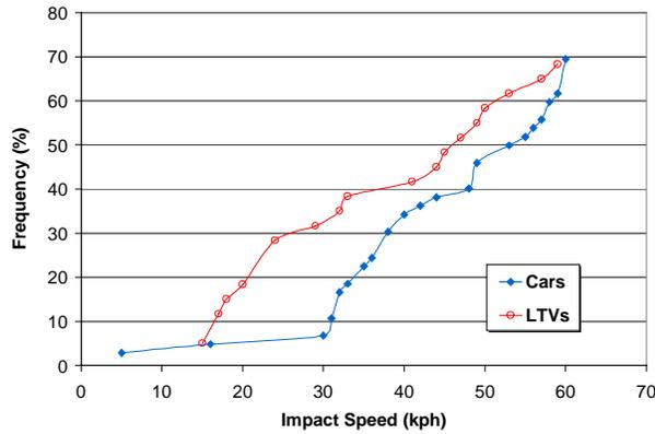
**Figure 7. Frequency of Severe Head Injury AIS 3 or Greater by Vehicle Type as a Function of Impact Speed**
