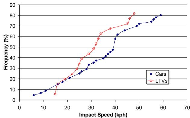
**Figure 9. Frequency of Severe Lower Extremity Injury AIS 3 or Greater by Vehicle Type as a Function of Impact Speed**
