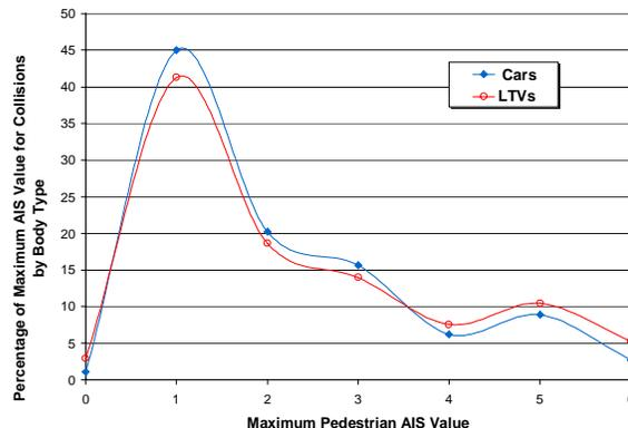
**Figure 5. Frequency of Maximum AIS Value by Vehicle Type**
