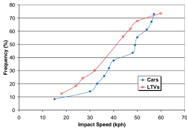
**Figure 8. Frequency of Severe Chest Injury AIS 3 or Greater by Vehicle Type as a Function of Impact Speed**
