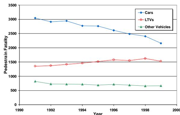
**Figure 3. Pedestrian Fatality Trend by Vehicle Type for Single Vehicle-Pedestrian Collisions**
