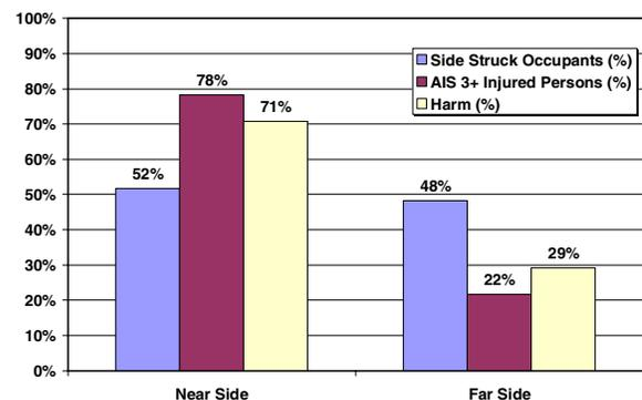
**Figure 2. Comparison of U.S. Near and Far Side Impact Injuries for 3-Pt Restrained Occupants**
