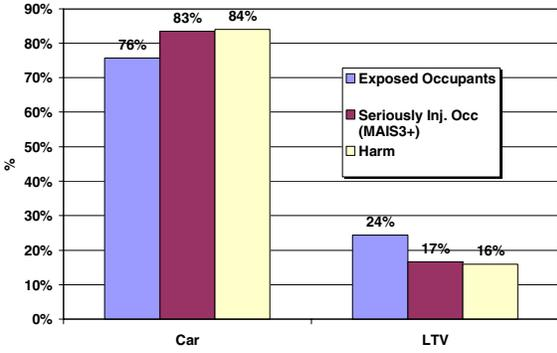
**Figure 6. U.S. Far Side Impact Injuries by Body Type of Struck Vehicle**
