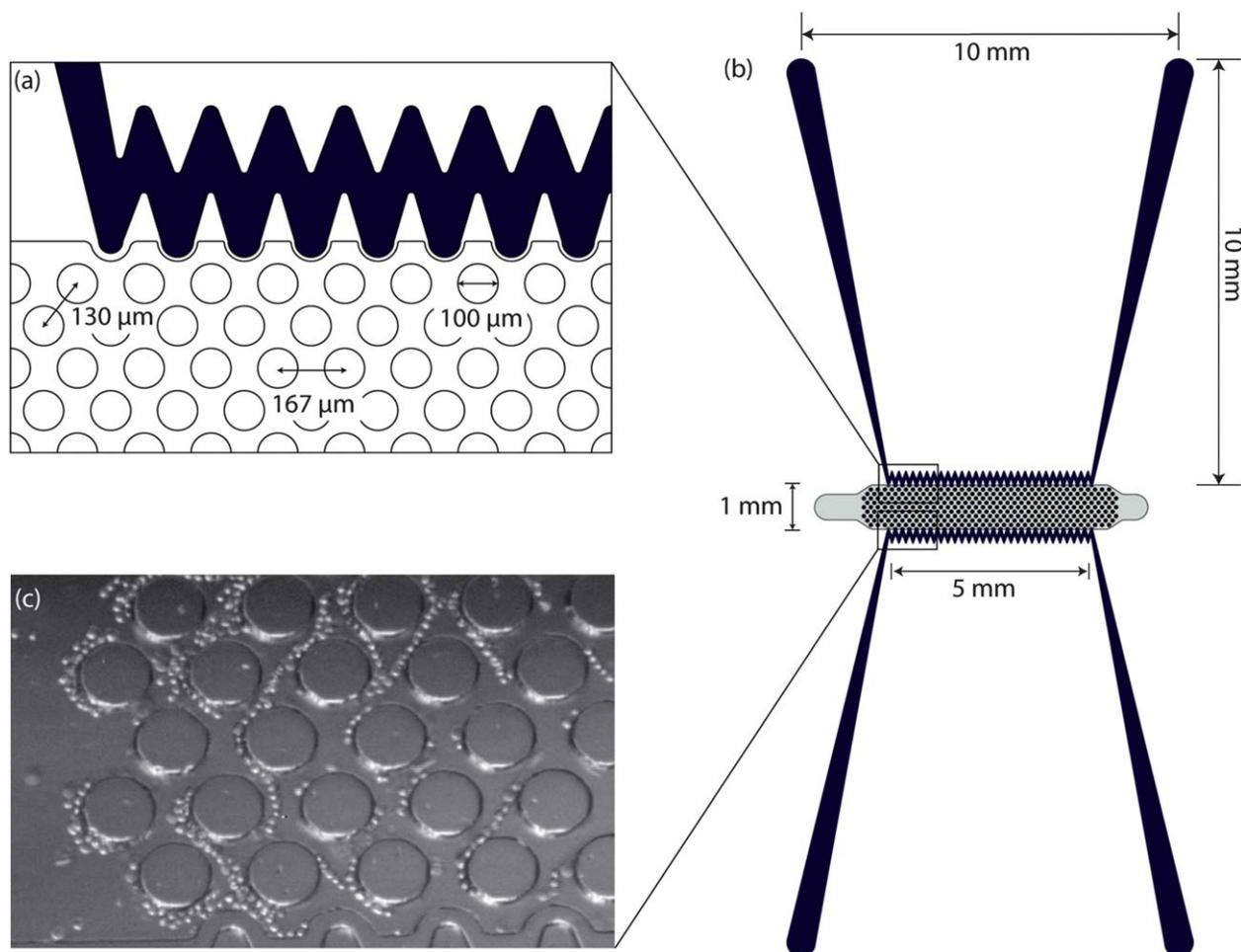
**Fig. 1** Top view schematic and dimensions of (a) a section of microchannels and pillars and (b) cDEP microdevice. (c) Trapped cells at 600 kHz and 129  $V_{\text{rms}}$ .
