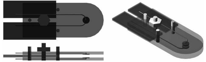
Fig. 1. Electroporation and impedance measurement device. Exposed liver lobe was placed between the two plate electrodes (10-mm diameter). Electrodes and insulating plates were held 4 mm apart by spacers inserted between the plates. Three pins that extended through both plates ensured concentricity of the electrodes (not to scale).
