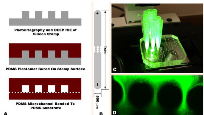
**Figure 2 : a) Fabrication process for creating microchannels. b) Schematic showing the top view of the channels with insulating pillars. c) Experimental setup for interfacing with microfluidic channels. d) Fluorescently labeled *A. xylinum* cells being controlled through a microchannel dielectrophoretic forces.**
