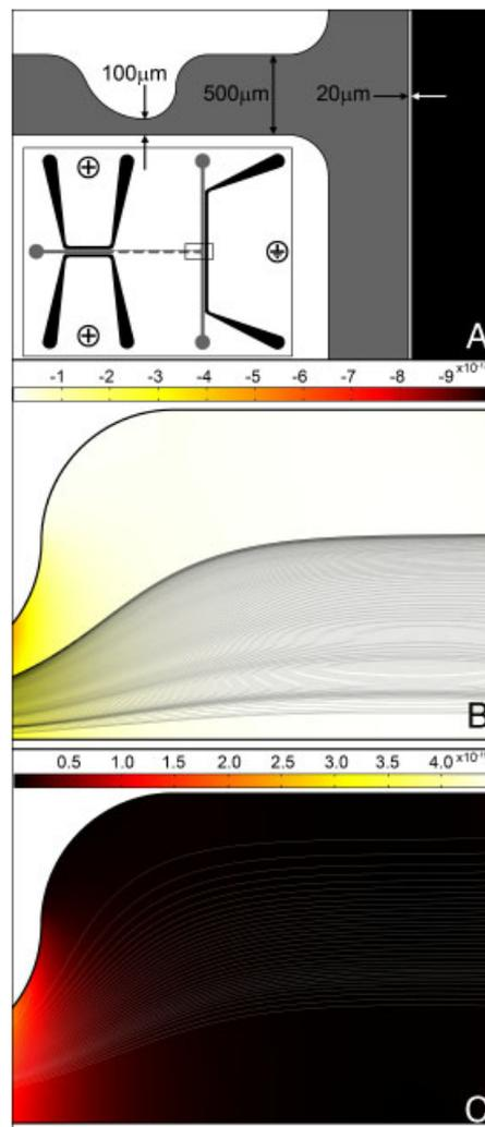
**Figure 1.** (A) Schematic of the low-frequency contactless DEP device. The fluid electrodes and sample channel are shown in black and grey, respectively. Particle-independent DEP vector ( $\text{EV}^2\text{m}^{-3}$ ) and particle trajectories for 200 MDA-MB231 cells at (B) 10 kHz and (C) 70 kHz. 84% of particles intersected the top of the channel in (C) indicating that a large number of cells will travel along the upper wall.
