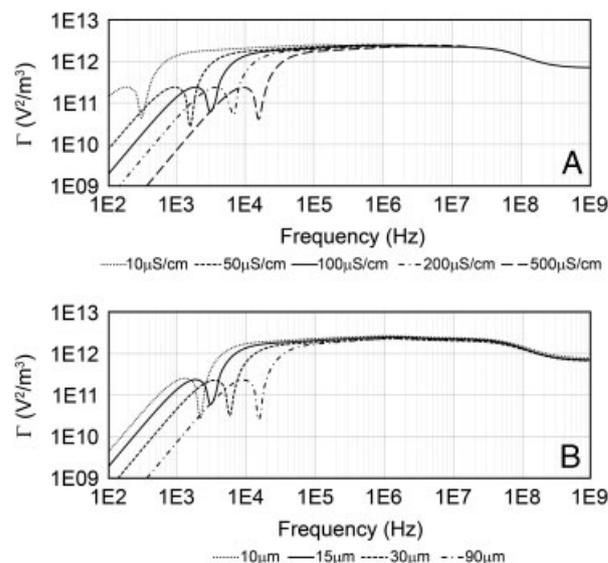
**Figure 3.** Parametric analysis of device performance varying (A) sample conductivity and (B) barrier thickness. Nominal values are: barrier thickness = 15  $\mu\text{m}$  and sample conductivity = 100  $\mu\text{S/cm}$
