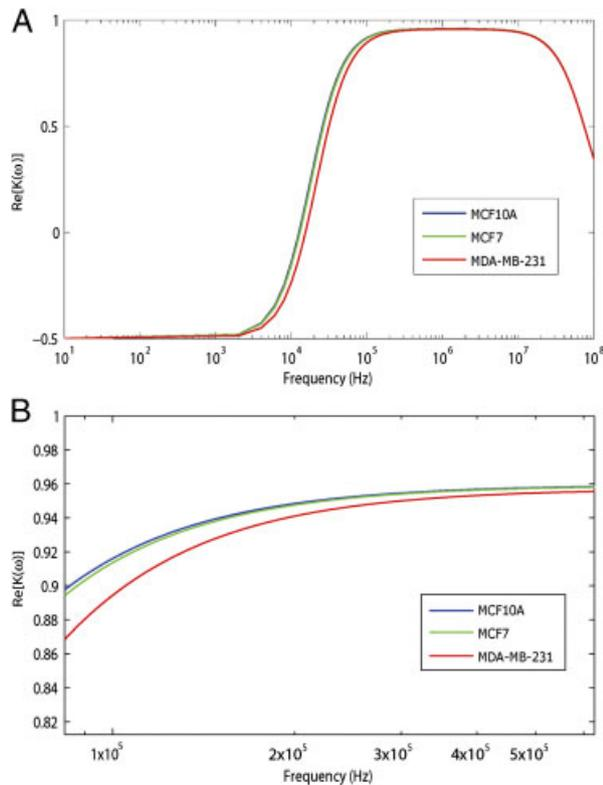
**Figure 3.** (A) The real part of the Clausius–Mossotti factor for MCF10A, MCF7, and MDA-MB-231 cells using estimated parameters in Table 1. (B) Zoomed in image of the curve at experimental frequencies.
