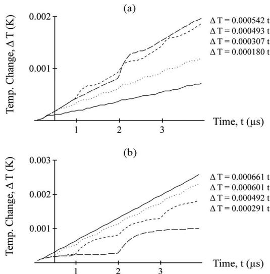
Fig. 6. Temperature changes predicted by the FEM at the center of the (a) skin and (b) fat for frequencies of 250 kHz (—), 500 kHz (- - -), 1 MHz (· · ·), and 2 MHz (-). Equations represent a linear fit to the data.
