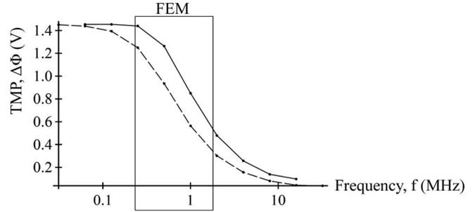
Fig. 4. Frequency  $f$  response of the TMP at the cell pole ( $\theta = 0$ ) for rectangular bipolar pulses (—) and sinusoidal waveforms (---). The box illustrates the frequency window implemented in the FEM.
