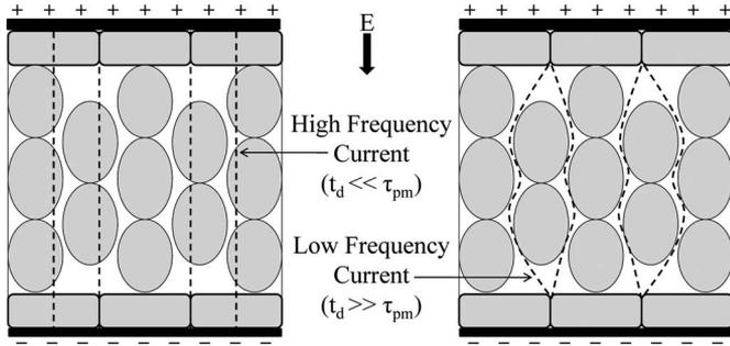
Fig. 1. Illustration of current pathways through epithelial layers and bulk tissue prior to the onset of electroporation. When the pulse duration  $t_d$  is much less than the plasma membrane time constant  $\tau_{pm}$ , current flows through both intracellular and extracellular spaces (left). In the case that  $t_d$  is much more than  $\tau_{pm}$ , current flow is restricted to the narrower extracellular spaces (right).
