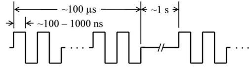
Fig. 2. Typical pulsing protocol for the proposed electroporation-based therapy. The total burst width of the high-frequency pulses ( $\sim 100$  to  $1000$  ns duration of single polarity) is on the order of hundreds of microseconds, the time delay in between bursts is on the order of seconds, and the total number of bursts can be adjusted.
