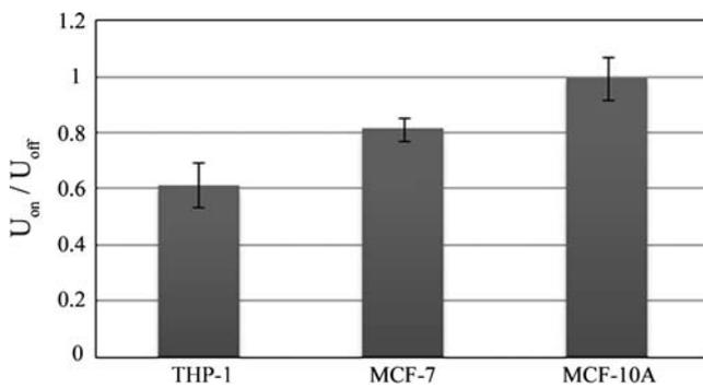
**Fig. 6** The normalized velocity of THP-1, MCF-7, and MCF-10A cells.  $U_{on}$  is the velocity of the cells while applying e-field and  $U_{off}$  is the velocity of the cells while the power is off
